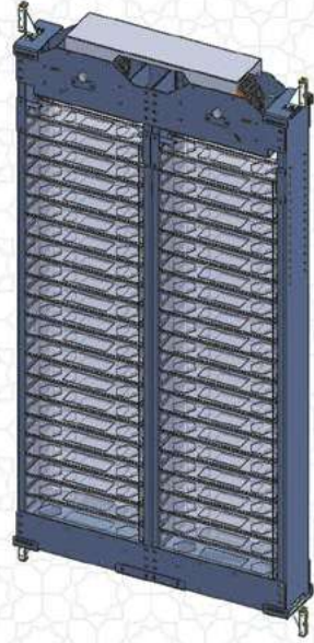
COUNTER WEIGHT SUSPENSION 2:1
